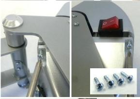
Install top half of Controller Housing and secure by screwing in 4x #6 x ½" Screws using #2 Phillips Screwdriver
