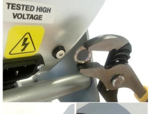
Install silver mounting ring onto new Circuit Breaker using Pliers, being careful not to scratch painted surface
