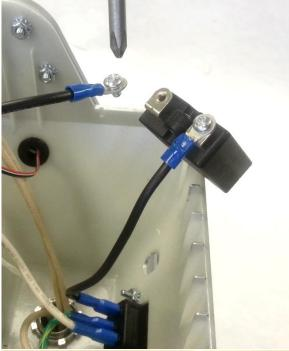
Transfer wires one at a time from old Circuit Breaker to new using #2 Phillips Screwdriver, noting terminal connections as shown
