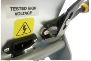
While holding old Circuit Breaker in place and being careful not to scratch painted surface, unscrew silver retaining ring using Pliers and remove old Circuit Breaker from housing
