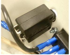
Insert new Circuit Breaker into housing with toothed locking washer as shown
